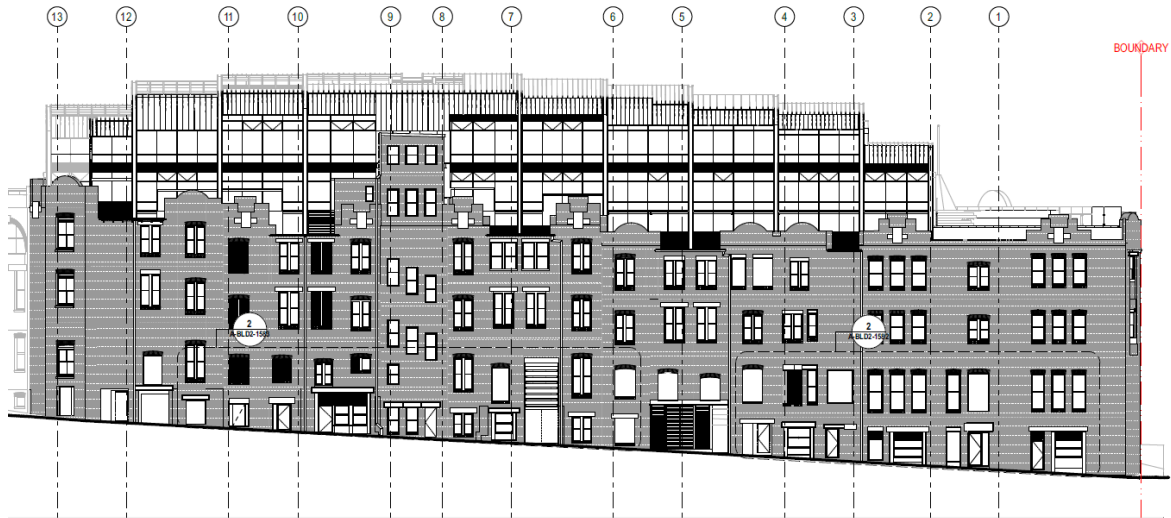
Figure 28: Proposed Foley Street shopfront details elevation
