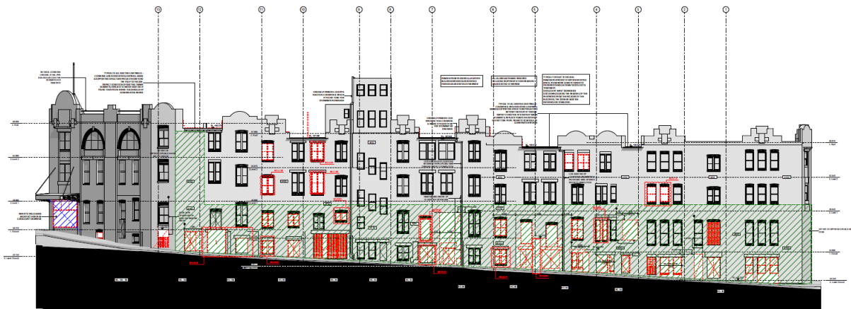
Figure 35: Proposed Foley Street demolition elevation
